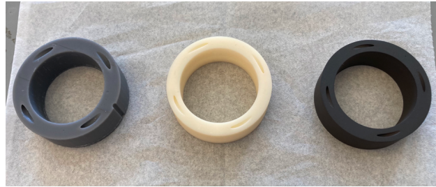
Fig. 2 The three types of prototyped diffusers. From left to right: low temperature SLA resin, Somos PerFORM, and black anodized aluminum. This figure by Braden Oh, et al. [3] is licensed under CC BY 4.0.
