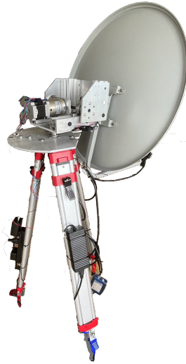
Fig. 11 Fully Integrated Alpha Prototype of the ACU
